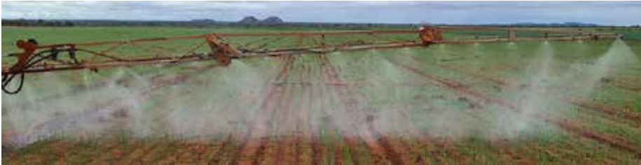
Figure 2. Spraying of the Nu-Film P added onion plot with a boom sprayer calibrated to 500l/ha during April 2022 near Swartwater, Limpopo province.
