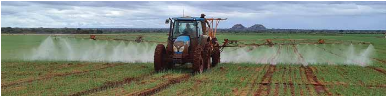
Figure 2. Spraying of the Nu-Film P added onion plot with a boom sprayer calibrated to 500l/ha during April 2022 near Swartwater, Limpopo province.
